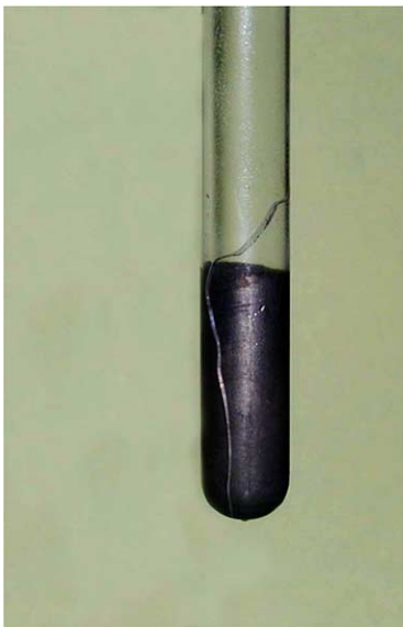
Fig. 3. A crack in a broken glass tube demonstrates the expansion of LBE during aging.
